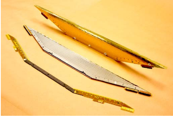
Fig. 9. Anode frame with wires ( front ); cathode frame with the Vernier foil ( middle ); completed drift chamber ( back )
