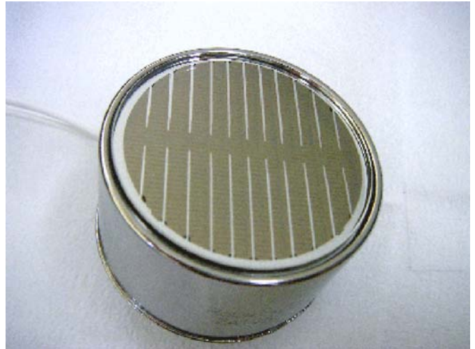
Fig. 12. Photomultiplier for the MEG LXe detector
